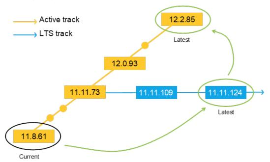
Upgrading from the latest LTS track to the active track: Start by upgrading to the latest version of your current LTS.
