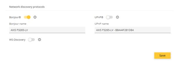
Why is this change introduced? To lower the attack surface of the device and increase the overall device security. How can it affect me? If you have third party software only using UPnP for device discovery, it will not work correctly with AXIS OS 12.1 or higher and users need to enable UPnP first on the Axis device.
