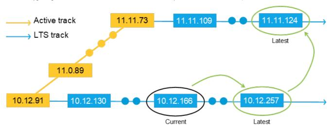
• Upgrading from an older LTS to two newer LTS versions: Upgrade to the intermediate LTS version first.
