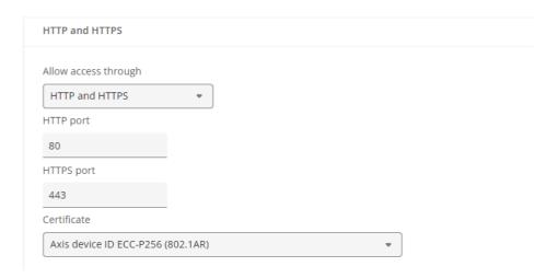
This default behavior is likely to change in order to increase overall default security and protect communication between the Axis device and the human user as well as applications. Axis has plans to change the default behavior so that HTTP communication will be disabled, and HTTPS-only communication is the only enabled protocol to be used in factory defaulted state.
