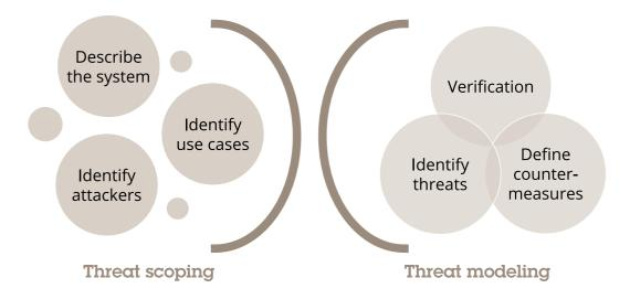
Focus during threat scoping is on finding and categorizing attackers we want to handle using a high-level description of the system. Preferably the description is done using a data flow diagram (DFD) since it makes it easier to relate the more detailed use case descriptions that are used when doing the threat model.
