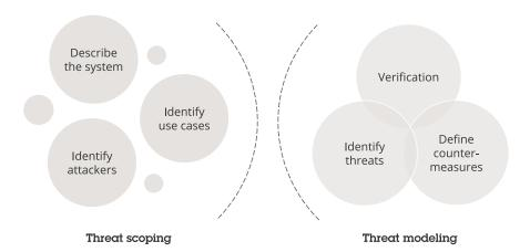
The focus during threat scoping is on finding and categorizing attackers we want to handle using a high-level description of the system. Preferably, the description is visualized as a data flow diagram (DFD) since it makes it easier to relate the more detailed use case descriptions that are used when creating the threat model.
