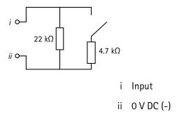
UL: Supervised inputs were not evaluated by UL for burglary use. Only door monitor and REX support supervision with end of line resistors.
