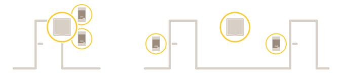
Each network door controller is an intelligent device that is easily mounted close to a door. It can power and control up to two readers.
