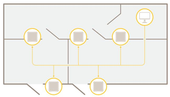
The network door controller can easily be connected to and powered by your existing IP network with no need for special cabling.
