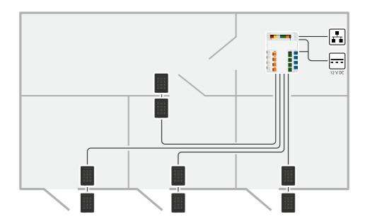
The network door controller can easily be connected to your existing IP network. Each network door controller can power and control up to 8 readers.
