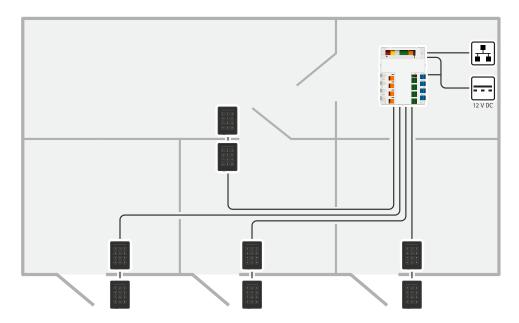
The network door controller can easily be connected to your existing IP network. Each network door controller can power and control up to 8 readers and 4 locks.
