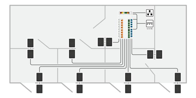
The network door controller can easily be connected to your existing IP network. Each network door controller can power and control up to 16 readers.
