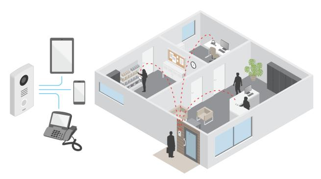
When you press the call button on an Axis door station, a call is initiated to one or more predefined recipients. When a recipient replies, a call is established. The voice and video is transferred through VoIP technologies.
