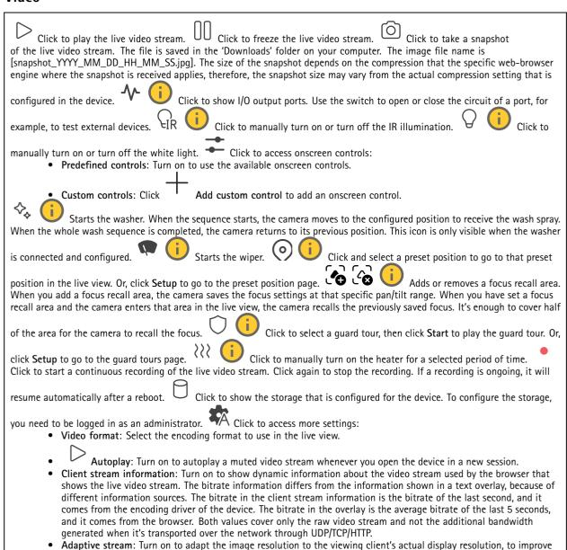
the user experience and help prevent a possible overload of the client's hardware. The adaptive stream is only applied when you view the live video stream in the web interface in a browser. When adaptive stream is turned on, the maximum frame rate is 30 fps. If you take a snapshot while adaptive stream is turned on, it will use the image resolution selected by the adaptive stream.
