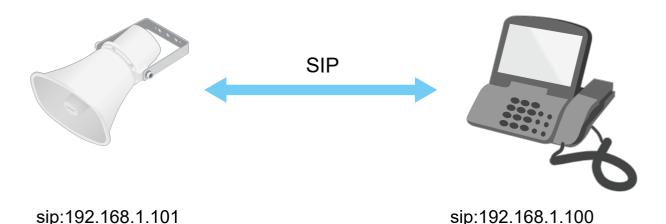
You can set up a SIP-enabled phone to call an audio device on the same network using a peer-to-peer SIP setup.
