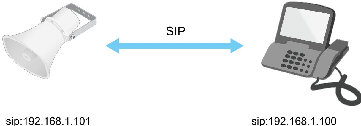
You can set up a SIP-enabled phone to call an audio device on the same network using a peer-to-peer SIP setup.
