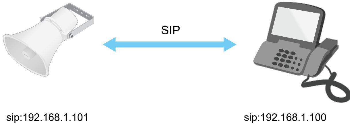
You can set up a SIP-enabled phone to call an audio device on the same network using a peer-to-peer SIP setup.
