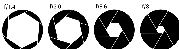
Examples of apertures for different f-numbers.
