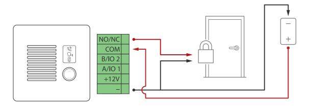
1. To check relay state, go to **System > Accessories** and find the relay port.
