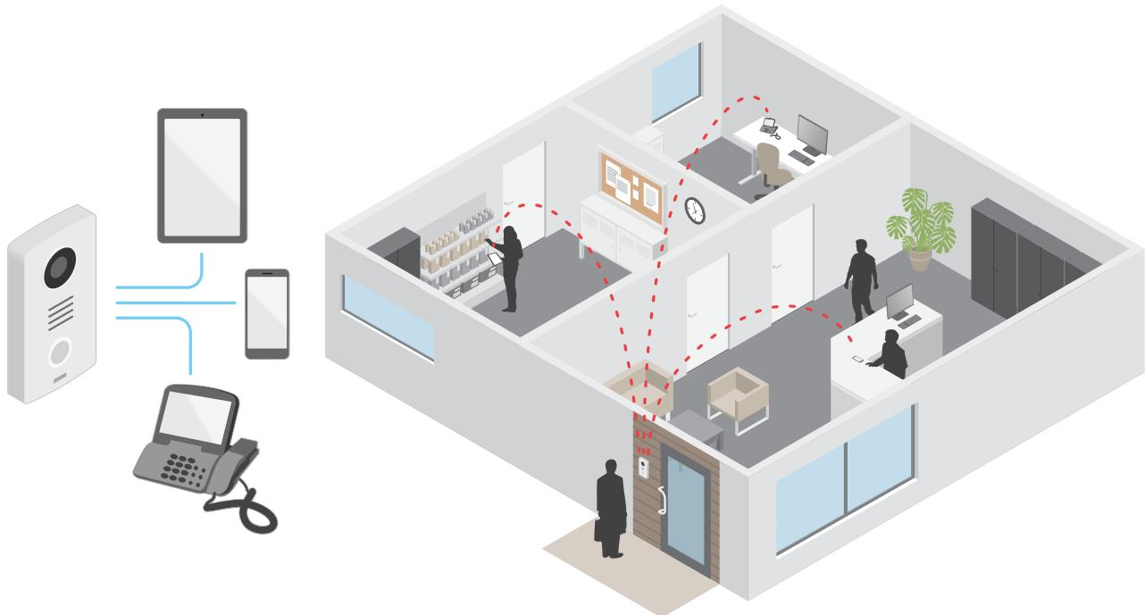
When you press the call button on an Axis intercom, a call is initiated to one or more predefined recipients. When a recipient replies, a call is established. The voice and video is transferred through VoIP technologies.
