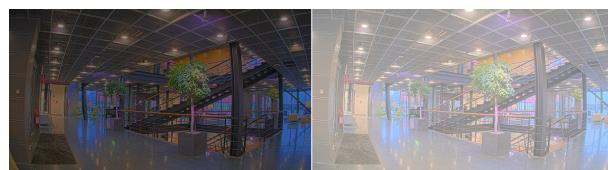
**Sharpness:** Use the slider to make objects in the image appear sharper by adjusting the edge contrast. If you increase the sharpness, it may increase the bitrate and the amount of storage space needed as well.
