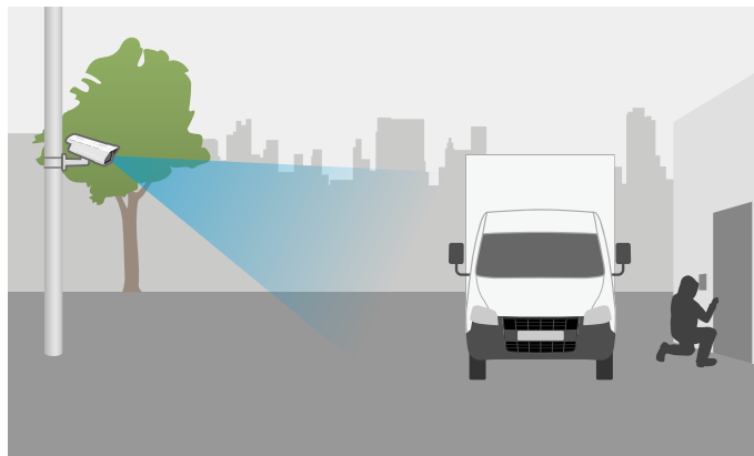
The camera view is blocked by an intentionally parked truck
