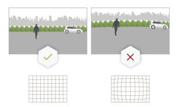
The image to the right is an example of barrel distortion. Barrel distortion is a lens effect where straight lines appear increasingly bent closer to the edges of the frame.
