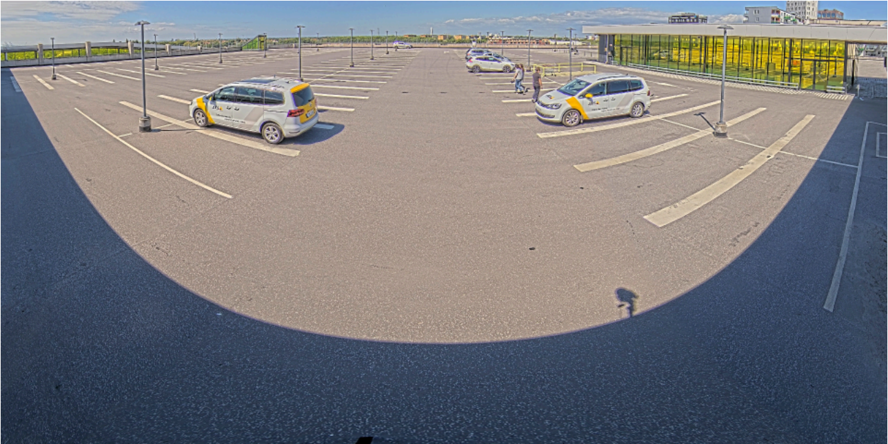
180-degree panoramic view snapshot taken with a multisensor camera with horizon straightening. The horizon is straight and vertical objects are vertical.
