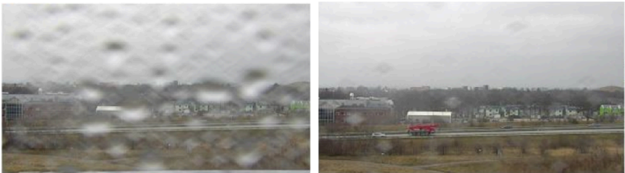
Snapshot from a camera's live view before and after speed dry has been activated.
