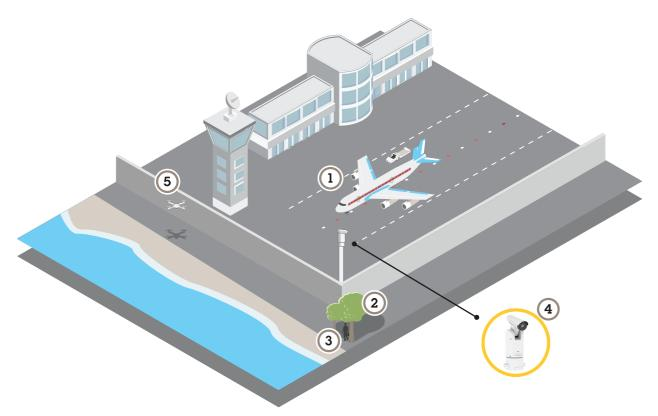
In difficult lighting conditions (2), the thermal camera can detect objects (3) that a visual camera cannot.
