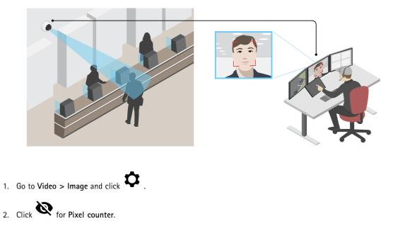
3. In the camera's live view, adjust the size and position of the rectangle around the area of interest, for example where you expect faces to appear.
