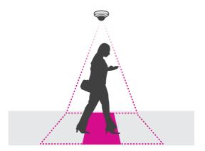
• Make sure the camera is facing straight down, in line with the ceiling.
