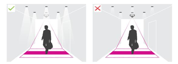
• Make sure that there are no continuously moving objects in the counting area. For example, do not install the camera above an escalator.
