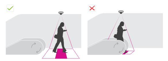
• Make sure there are no moving objects interfering in the counting area. For example, do not install the camera too close to a door.
