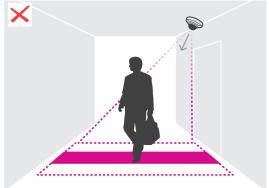
• If you install the application before you install the camera, you can use the counting area indicated in the live view to position the camera. The counting area should go from left to right, perpendicular to the path where people cross.
