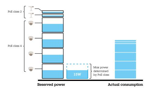
The power requested by each device is determined by the PoE class. The switch can power 4 PoE class 4 devices and 2 PoE class 2 devices. The total power requested is  $(4 \times 30) + (2 \times 7) = 134$  W. The actual power consumed is  $(4 \times 15) + (2 \times 5) = 70$  W. In this way, all connected devices are guaranteed enough power and the priority is less important.
