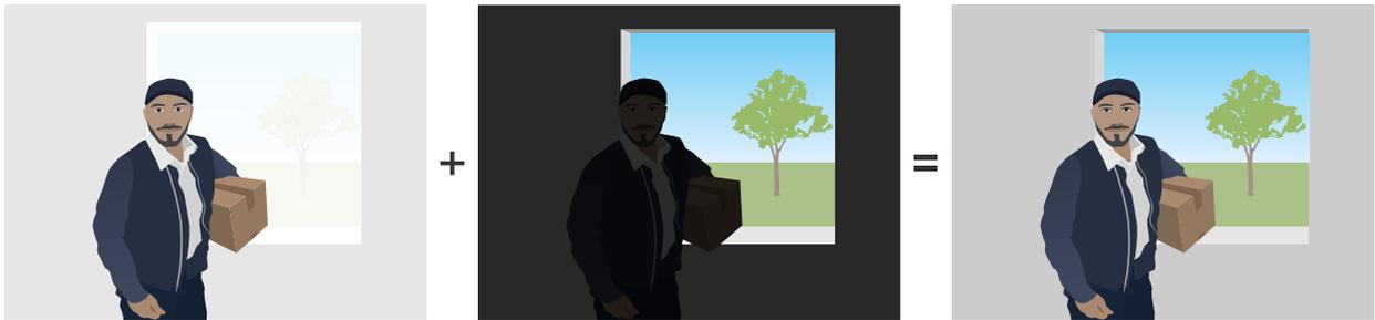
*The first two images show how the dynamic range in the monitored scene causes parts of the image to be overexposed or underexposed. In the third image, WDR dynamic capture has been used, resulting in a balanced image with all areas visible.*
