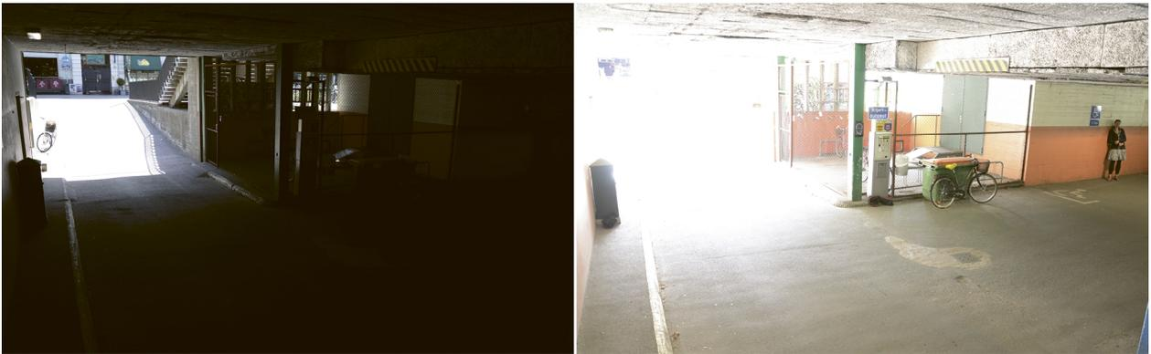
*A typical surveillance scene with a wide dynamic range: a parking garage interior with entrance. The two images were taken using different exposure times, shorter for the image to the left, and longer for the image to the right.*
