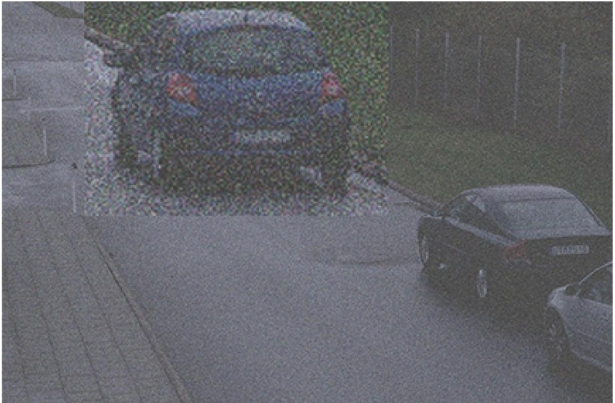
*Example of a dark scene where the gain function makes the scene brighter, but also results in image noise.*
