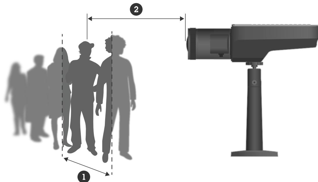
*Having a larger depth of field means that objects appear sharp at a larger range around the focal point.*
