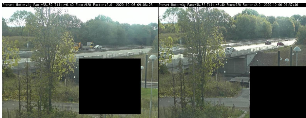
An original privacy mask and how the privacy mask, after some time, has drifted.
